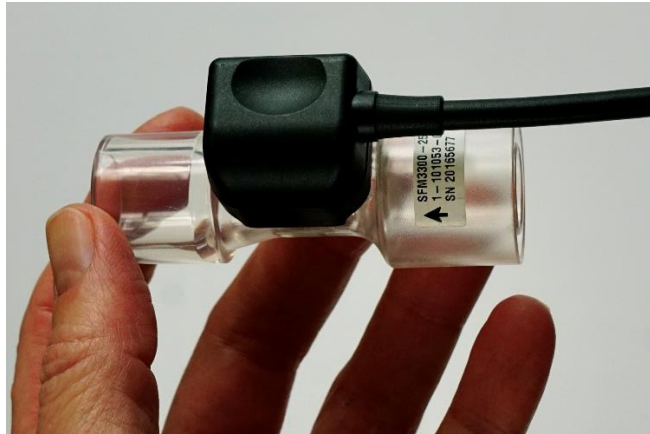
FIGURE 12-F: FLOW SENSOR CONNECTION TO FLOW SENSOR CABLE
