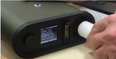
Insert ventilator tube into ventilator gas outlet
