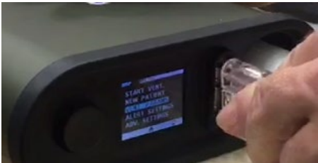
Insert the connector of the measurement and control tubes
